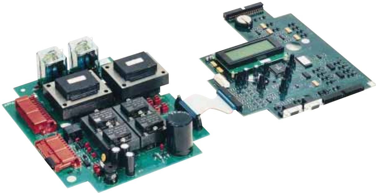
Fig.10 Microprocessor Power and Logic PC Boards.
